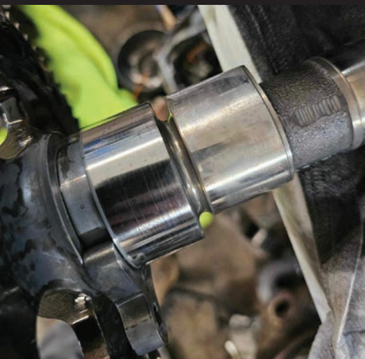
The camshaft and other major components on Kane's heavy-duty pickup truck were still in spec after 500,000 miles (804,672 km) of hard use.
